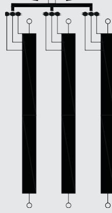
Setting for star transformer
